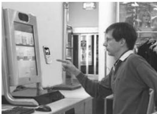
A camera based **hand tracker** detects hand gestures. It recognizes the position of the finger tip, which can be used for pointing at or for moving virtual objects represented with the stereoscopic display. The test person in front of the screen is able to touch, pick and turn the three-dimensional objects as if they were real without any further support of a stylus, glove or the like (virtual 3D touch screen).
