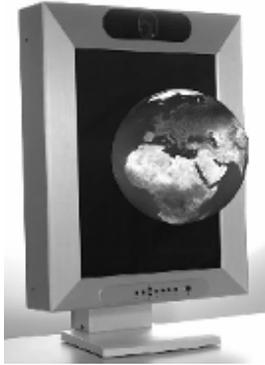
The Fraunhofer HHI **3D Kiosk system** offers simple intuitive handling as it presents any kind of object in a virtual manner on a large screen in photorealistic 3D quality (1600 by 1200 pixels; 21.3" screen). 3D-objects seem to float in front of the display for which no further technical additive like 3D-glasses or -helmet is necessary.
